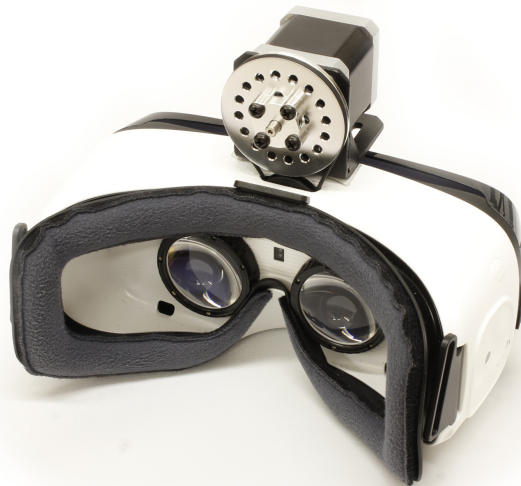
Fig. S2. A conventional near-eye display (Samsung Gear VR) is augmented by a gaze tracker and a motor that is capable of adjusting the physical distance between screen and lenses.
